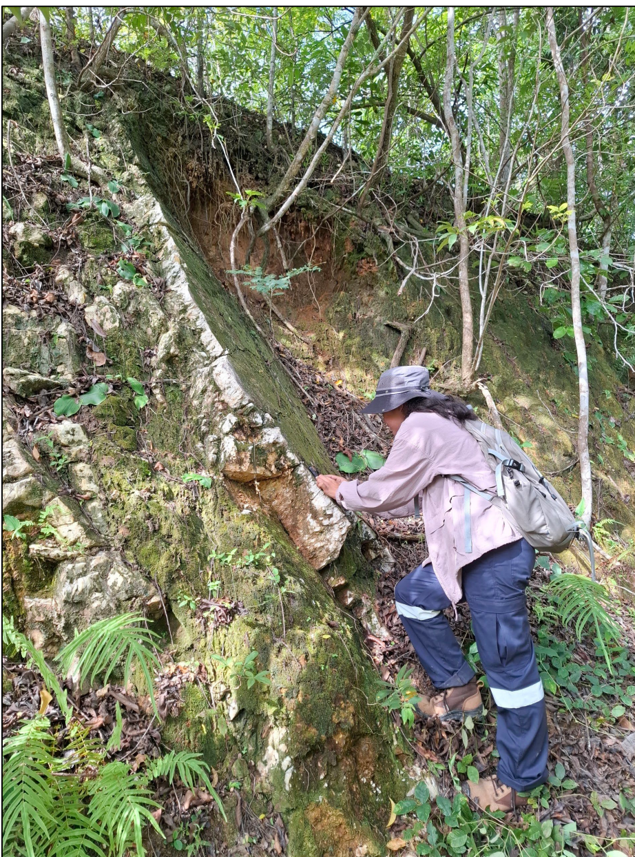
Figure 4: Photograph of massive and stockwork quartz veins located 55m east of the collar of 26DDCM007. The massive vein strikes 055° and dips 60° NW. Channel rockchip sample assays across this outcrop are pending and at this stage the gold content is unknown.
