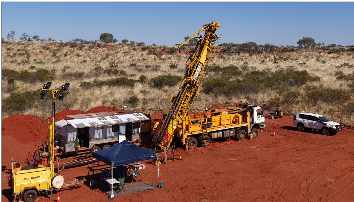
Figure 1. Diamond drilling at Khya, West Arunta Project
