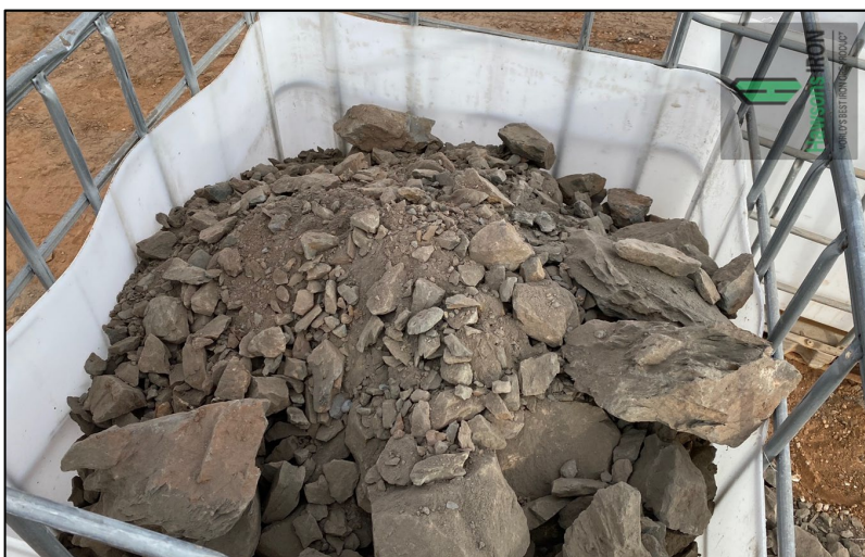
Figure 5: RCFO23015 drillhole sump and an example of the sample recovered
