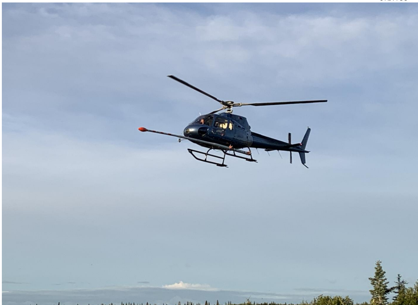
Figure 2: Commencement of geophysics survey (magnetics / radiometrics) showing Astar and survey boom
