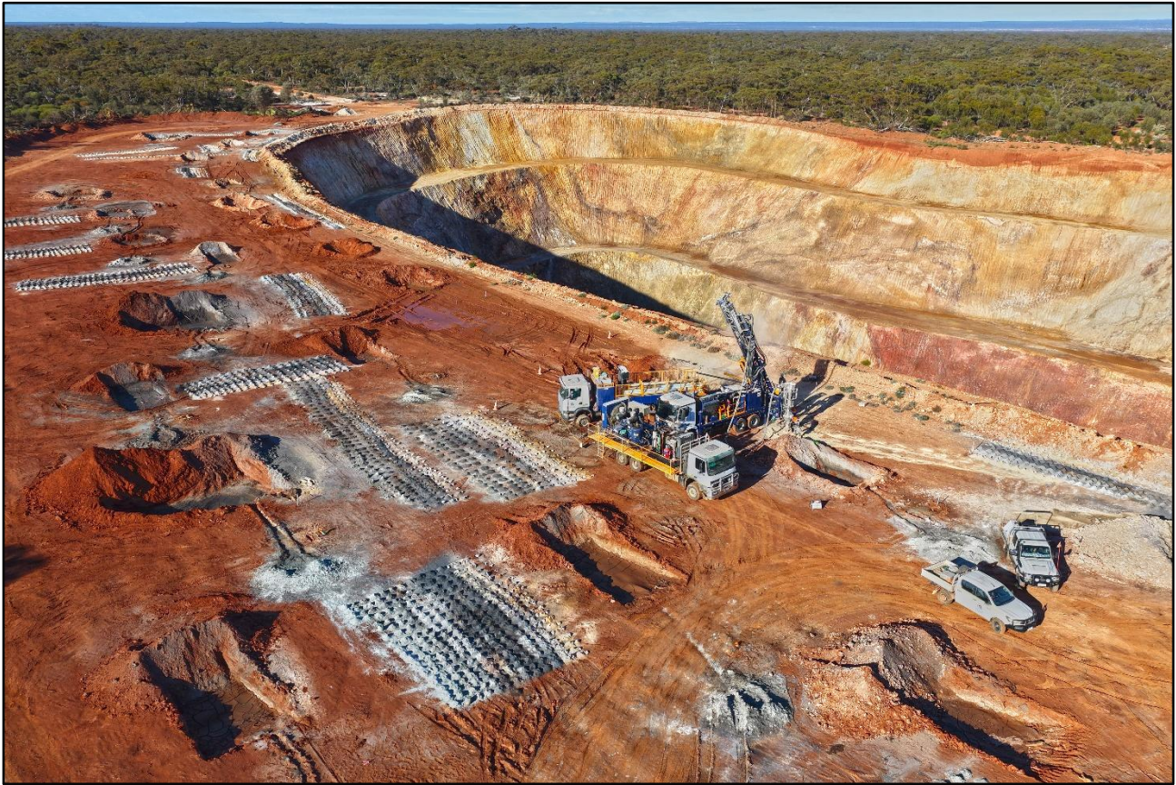
Figure 3 – Boorara Project – RC drilling looking south-west - Resource defining drilling – Boorara Open Pit in the background
