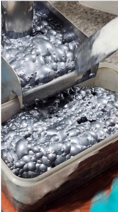
Figure 5: Flotation Testwork on Maronan Silver Lead samples being conducted at AMML Lab in Gosford (ASX: MMA 21 July 2026)
