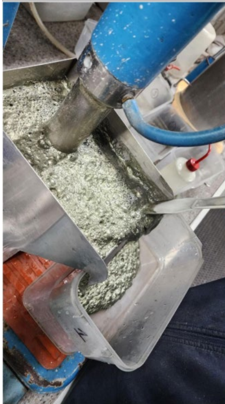
Figure 6: Flotation Testwork on Maronan Copper- Gold samples being conducted at AMML Lab in Gosford (ASX: MMA 21 July 2026)
