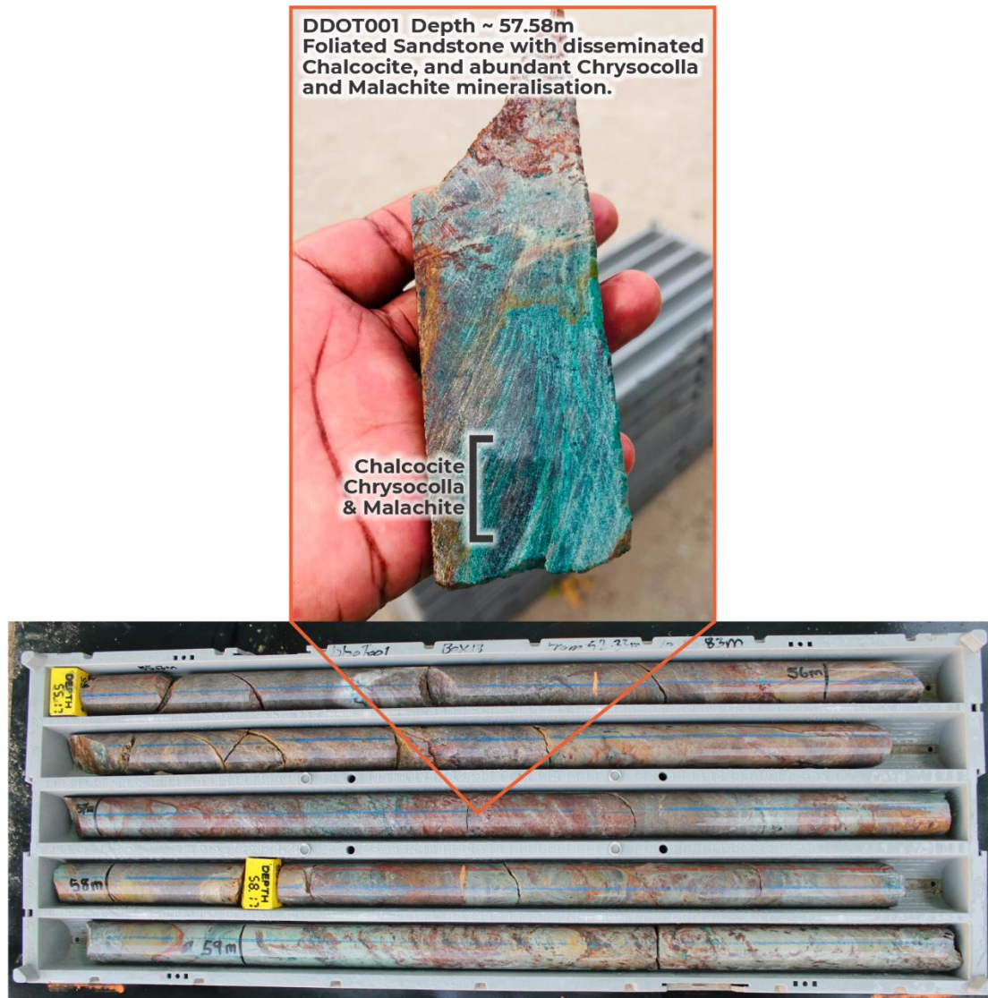
Figure 5 - DDOT001 Core from 52.33m to 59.83m, showing a selection of mineralised drill core from ~57.58m, with the visually identified copper minerals annotated. Refer to Appendix A for details.
