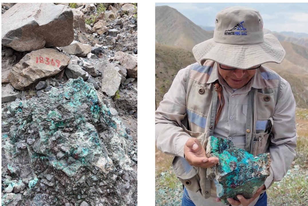
Figure 3: Cinto rock geochemistry. LHS (located proximate to Channel 7, sample 18369, taken across mineralisation in brecciated andesitic tuff exposed by gully erosion. Sample length 1.1m. Assay results: Au 0.535 g/t, Ag 25 g/t, Cu 8.7%, Mo 1 ppm, Pb 283 ppm, Zn 873 ppm 4 , RHS (located proximate to drill
