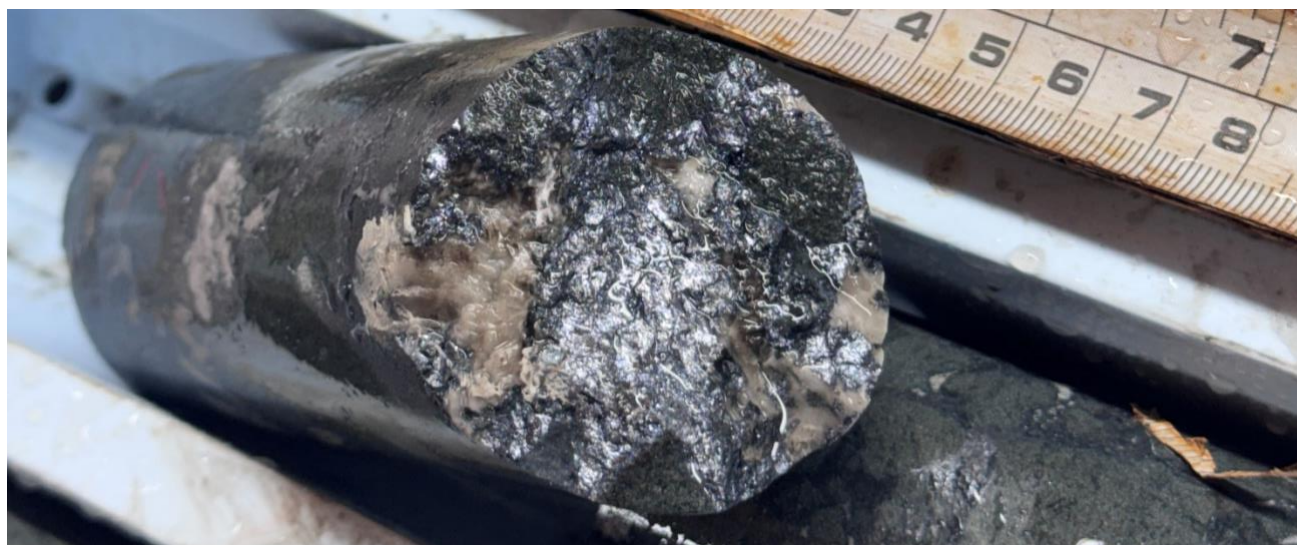
Figure 7 - Photograph of NQ2 diameter drill core displaying coarse grained chalcocite mineralisation from between 175.4 and 179.3m in drillhole DAN26036.
