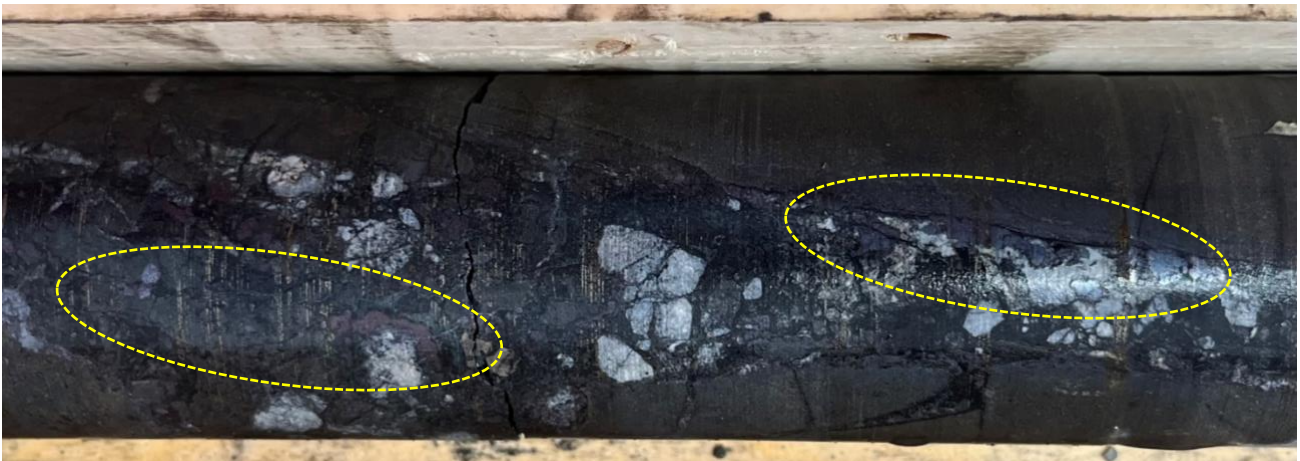
Figure 9 - Photograph of vein and breccia cement hosted chalcocite mineralisation that characterises the sulphides at 81m in DAN26047. Yellow dashed circles outline the bornite and chalcocite mineralisation. Drill core is NQ2 diameter.
