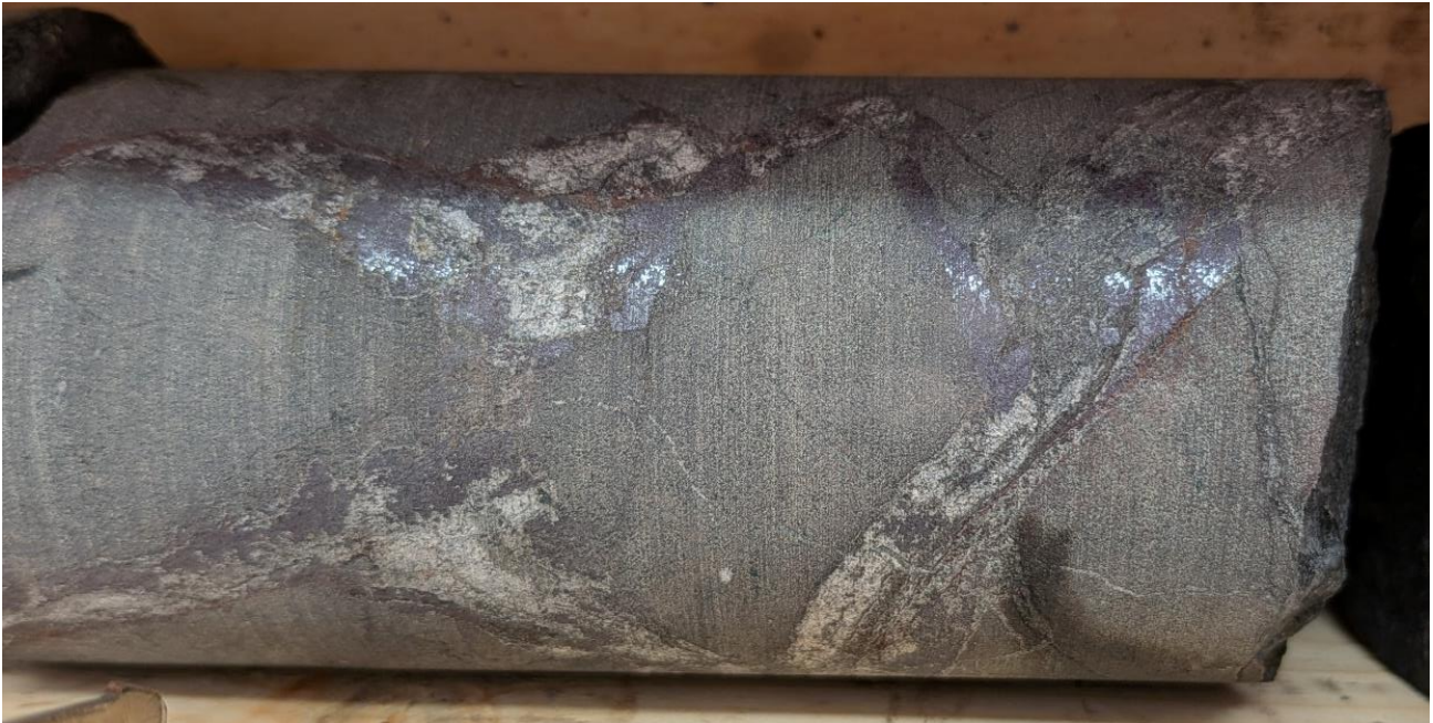
Figure 8 - Photograph of vein and breccia cement hosted chalcocite mineralisation that characterises the sulphides between 76m and 80m in DAN26047. Drill core is NQ2 diameter.
