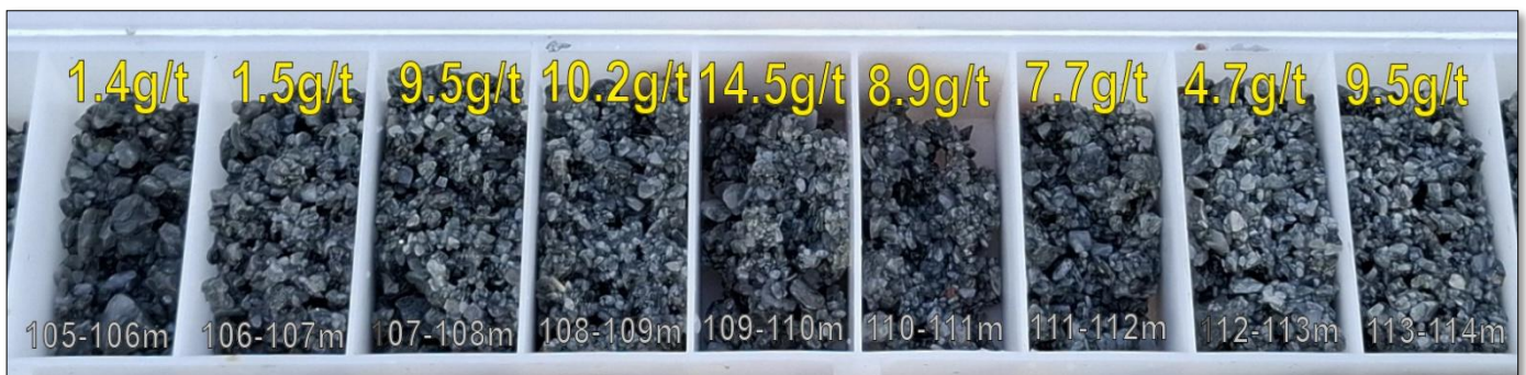
Figure 3: CZRC057 chip tray demonstrating the consistency in high-grade gold mineralisation from 105 metres to 114 metres (down-hole).
