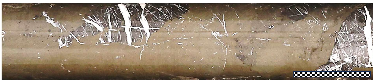
Figure 6. CD26-013 at 352.7m; massive sulphides with clasts of unmineralised shale and white carbonate veins. Scale bar approx. 5cm
