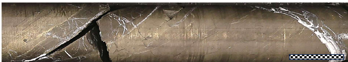
Figure 3. CD26-009 at 194.7m; massive sulphides. The darker sulphides are predominantly pyrite, the yellow green to brassy-yellow sulphide is chalcopyrite, with white carbonate veins. Scale bar approx. 5cm
