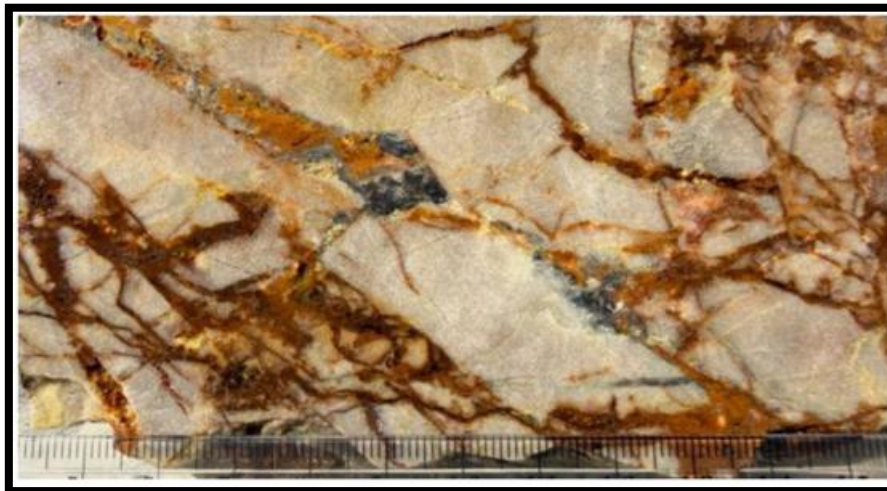
Figure 6. Silicified and brecciated rhyolite, Rock Chip sample 106064, lab certificate #TV26251464
