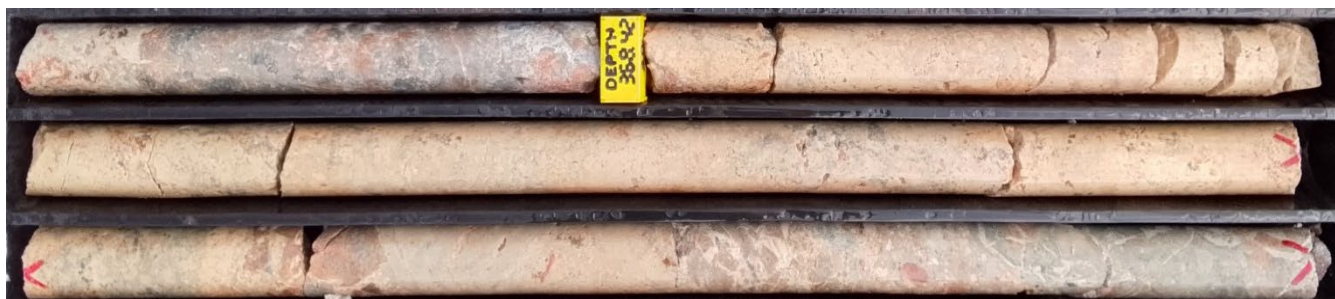
Figure 3 – 26NH023 ~368m to 370.5m depth apatite-rich calcite carbonatite interval bound on either side by clast supported carbonatite breccias.
