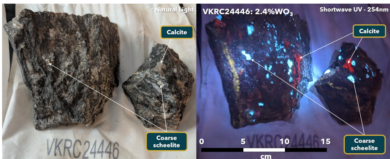
Figure 1; Photo of float sample from Terrell Project returning 2.4%WO 3 . Note extremely large and coarse scheelite crystals evident under shortwave UV light.
