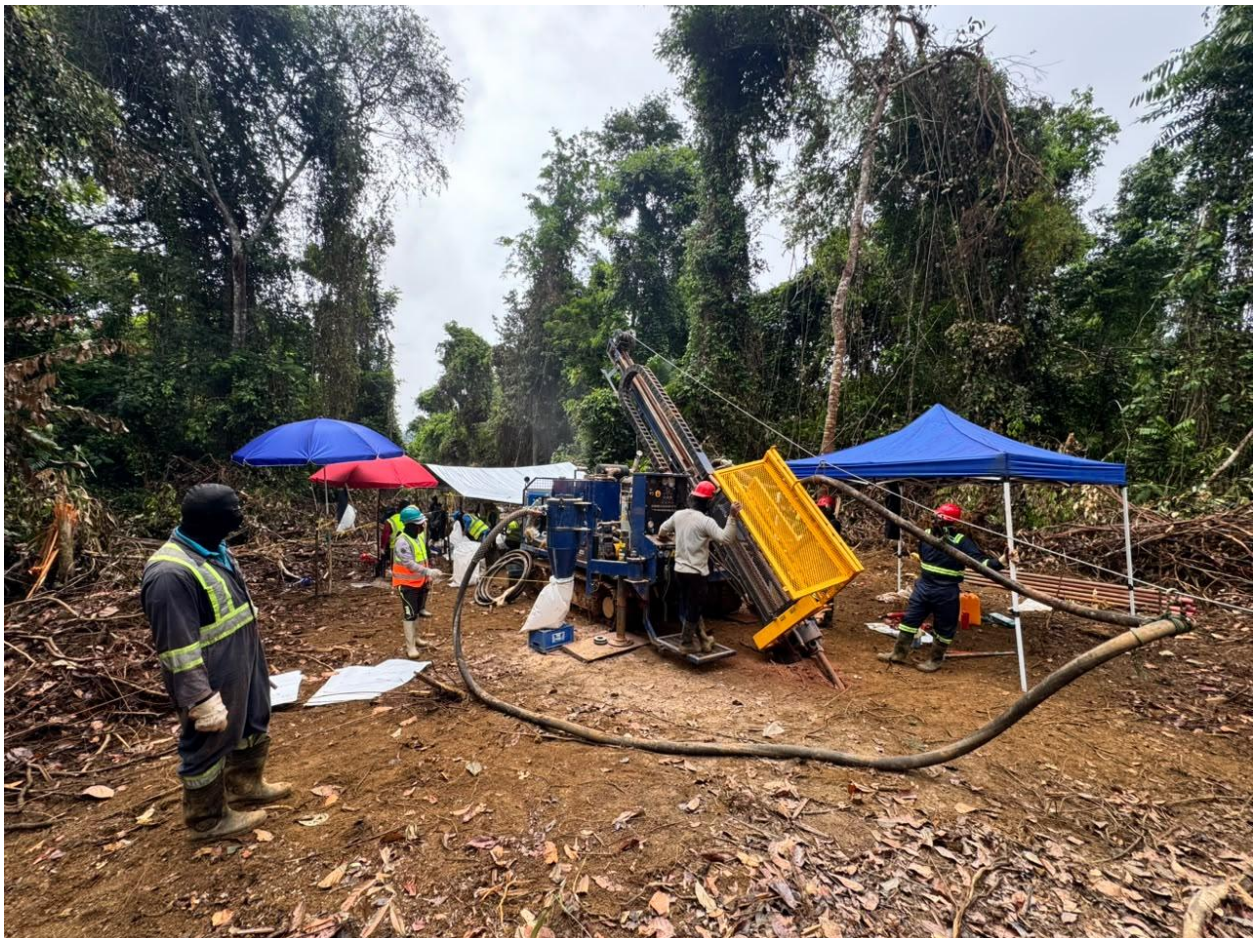
Figure 3: RC Drill Rig in operation at SOKO as part of 15,000m Phase I program.
