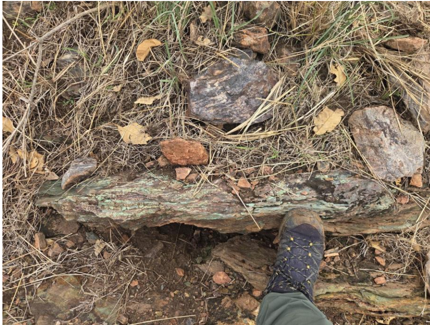
Figure 6: Copper Oxide mineralisation developed continuously along a schistose ledge in outcrop.
