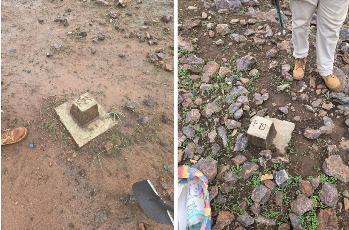
Figure 9: Monumented concrete collars of historical drill holes F23 (left) and F19 (right), located during the site visit.
