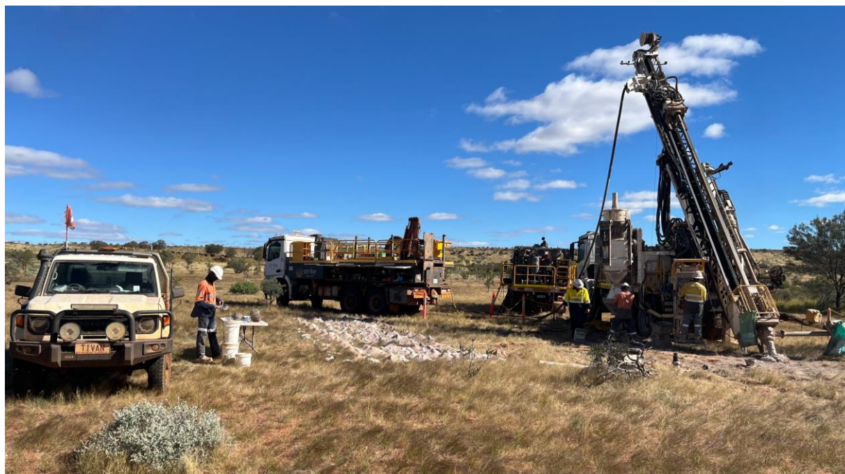
Figure 9: Low disturbance RC drilling at the Sandover Fluorite Project
