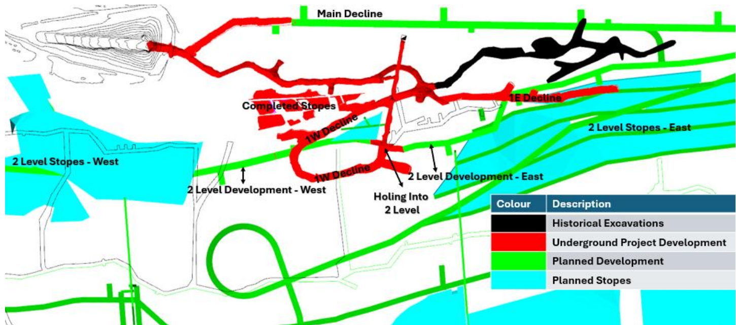
IMAGE 4: QALA SHALLOWS UNDERGROUND DEVELOPMENT WITH EXISTING WESTERN STOPING AREAS NOW ACCESSIBLE FOLLOWING 2 LEVEL BREAKTHROUGH VIA 1 WEST (1W) DECLINE
