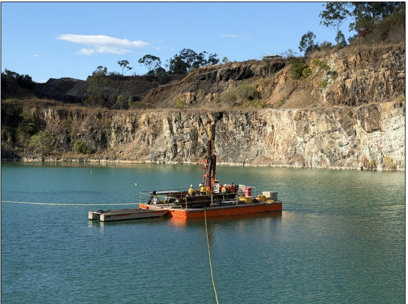
Figure 5: Diamond rig drilling beneath the existing open pit from a barge at the Mt Chalmers project.
