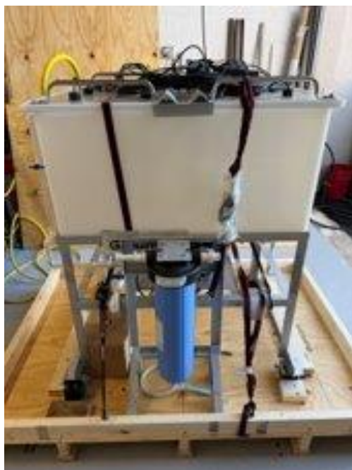
Figure 2: View of the 5 –10 gpm Fe removal unit boxed for transportation to Green River
