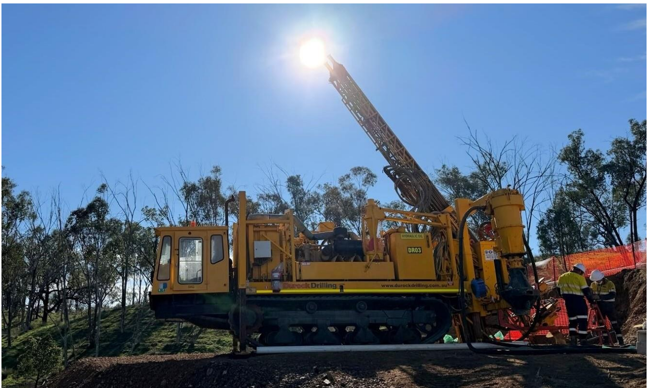
Image 1: RC Drilling Rig on site at Red Mountain Mining's Armidale Antimony-Gold Project in NSW, Australia
