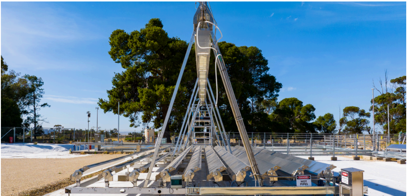
Sparc Hydrogen's concentrated solar reactor array at Roseworthy, South Australia.
