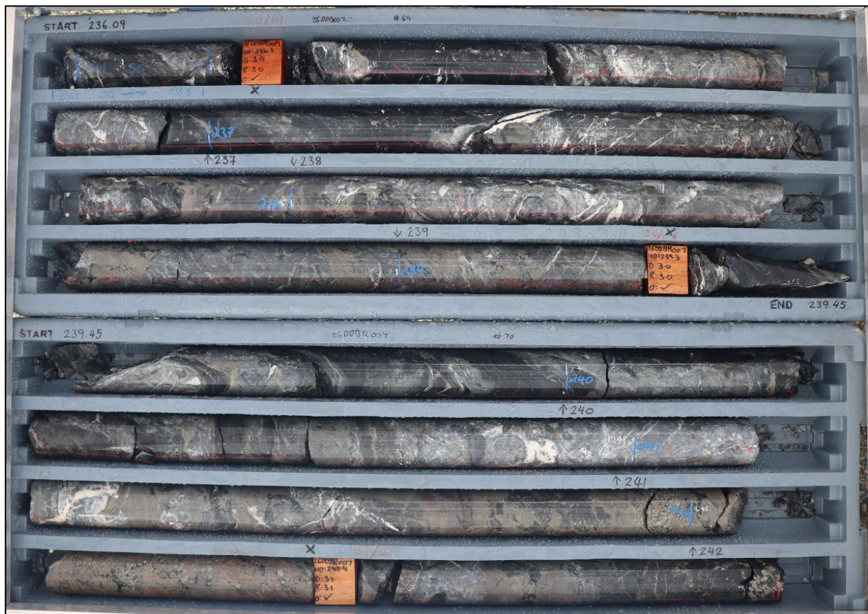
Figure 4: 26DDBR007 semi-massive sphalerite-pyrite-quartz zone within an interval of 12m at 0.5g/t Au, 6g/t Ag, 8.2% Pb+Zn & 0.1% Cu from 233m.
