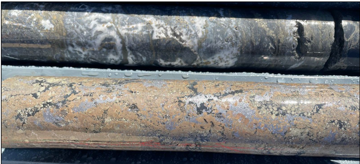
Figure 1: 26DDBR007 high-grade massive sulfide drill core, sphalerite (brown), galena (metallic), pyrite (bronze cubes) from 242.1m to 242.4m within interval 1.4m at 0.7g/t Au, 16g/t Ag, 22.6% Pb+Zn and 0.1% Cu from 241m.
