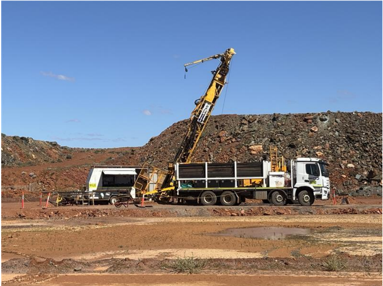
Figure 3: Diamond drill rig on first pad at Boomerang gold deposit
