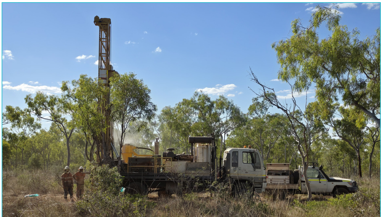
Figure 2: Reverse Circulation drilling at the Barkly Project.
