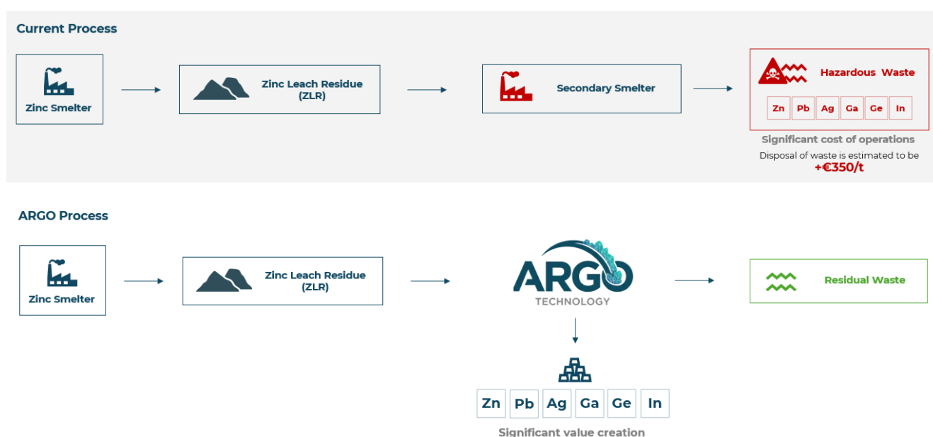
Figure 1: Schematic of the ARGO technology compared to the current process
