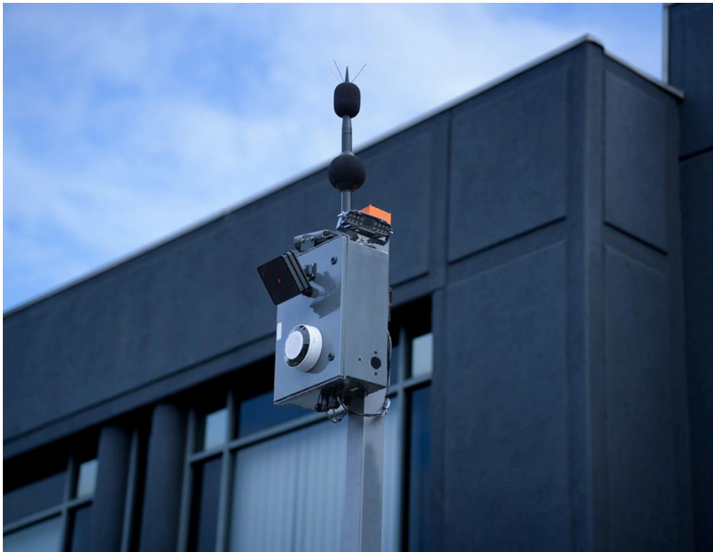
A fixed multi-sensor unit pairing cameras with acoustic sensors.
