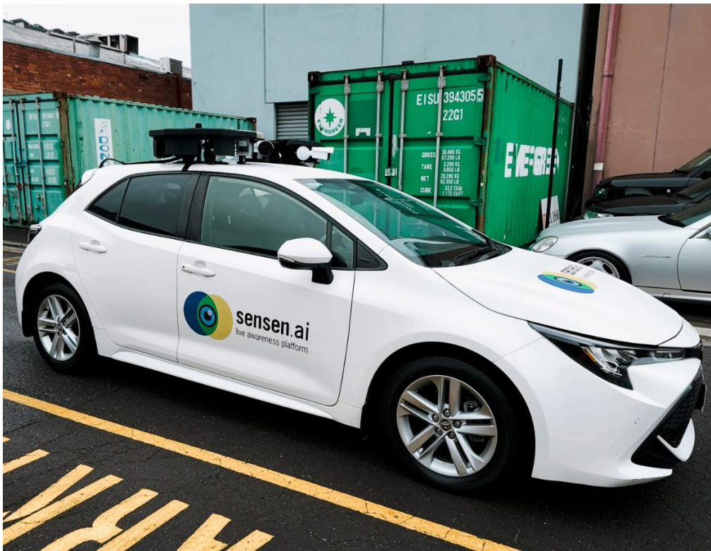
SenFORCE vehicle. The roof-mounted camera bar brings mobile enforcement to standard fleet cars.
