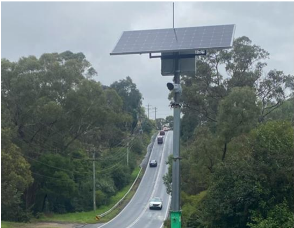
A solar-powered fixed pole monitoring a regional road corridor.
