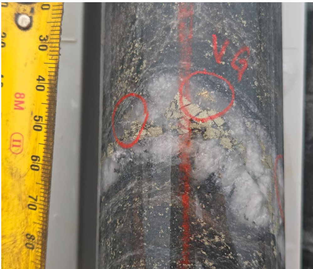
Figure 2: Visible gold in hole 26TBRD010 within a broad zone of shearing and associated with chalcopyrite, pyrite, albite and magnetite (assays pending).
