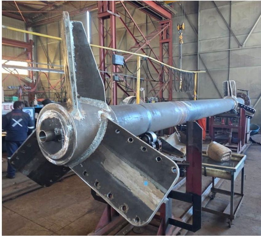
Image 5: Tank Agitators being manufactured (July 2026)
