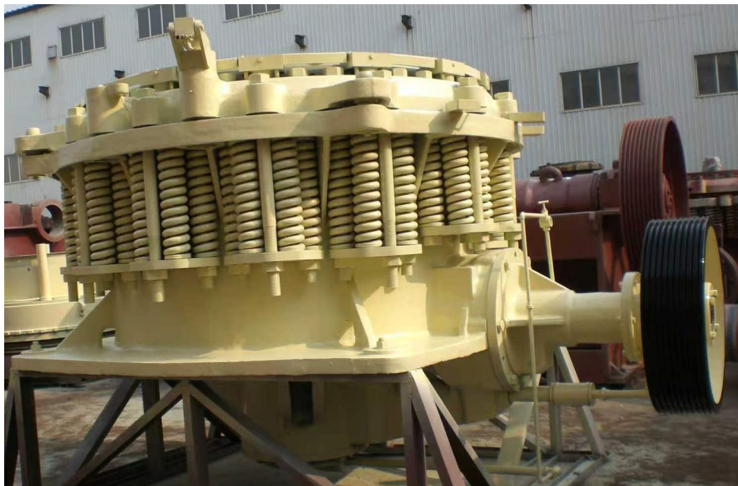
Image 6: Secondary Cone Crusher ahead of transit to Lake Johnston
