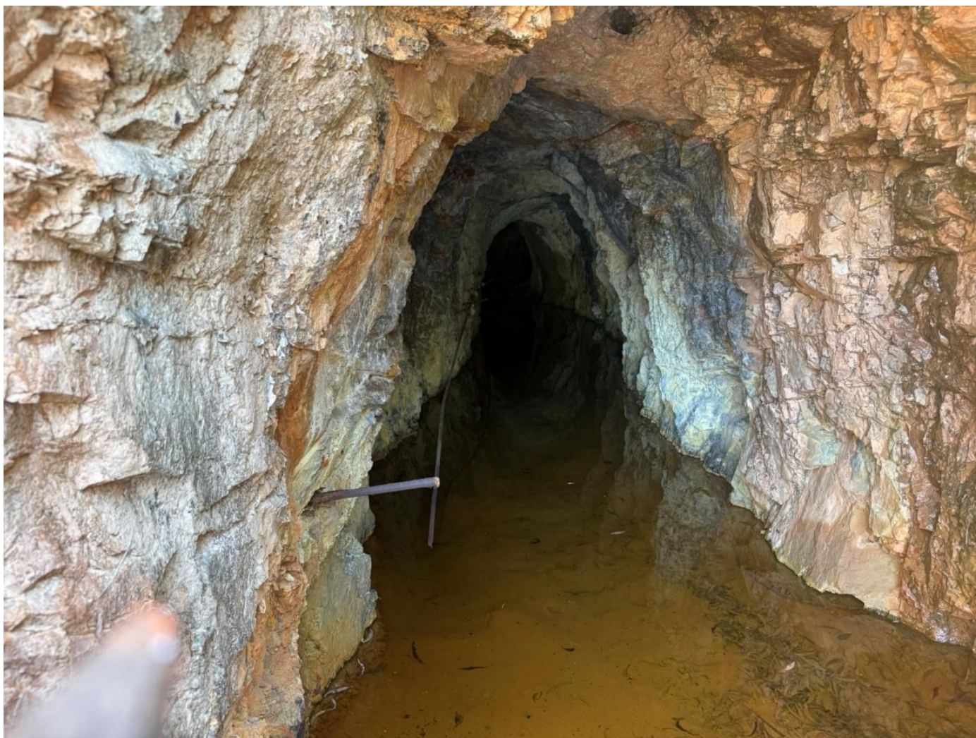
Figure 5: Historic mine haulage adit at the Elizabeth Mine (new workings) which drives through the vein perpendicularly. A sample traverse of 8.5m at 1.08% Cu and 0.44% Sn was taken at the far end of this adit.
