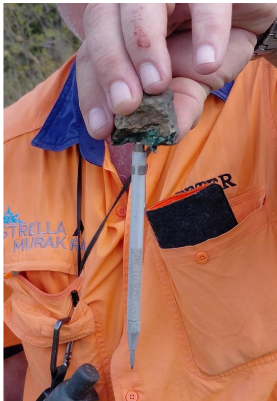
Figure 11: Portion of sample ESR006489, showing strong magnetic attraction to magnetic scribe.
