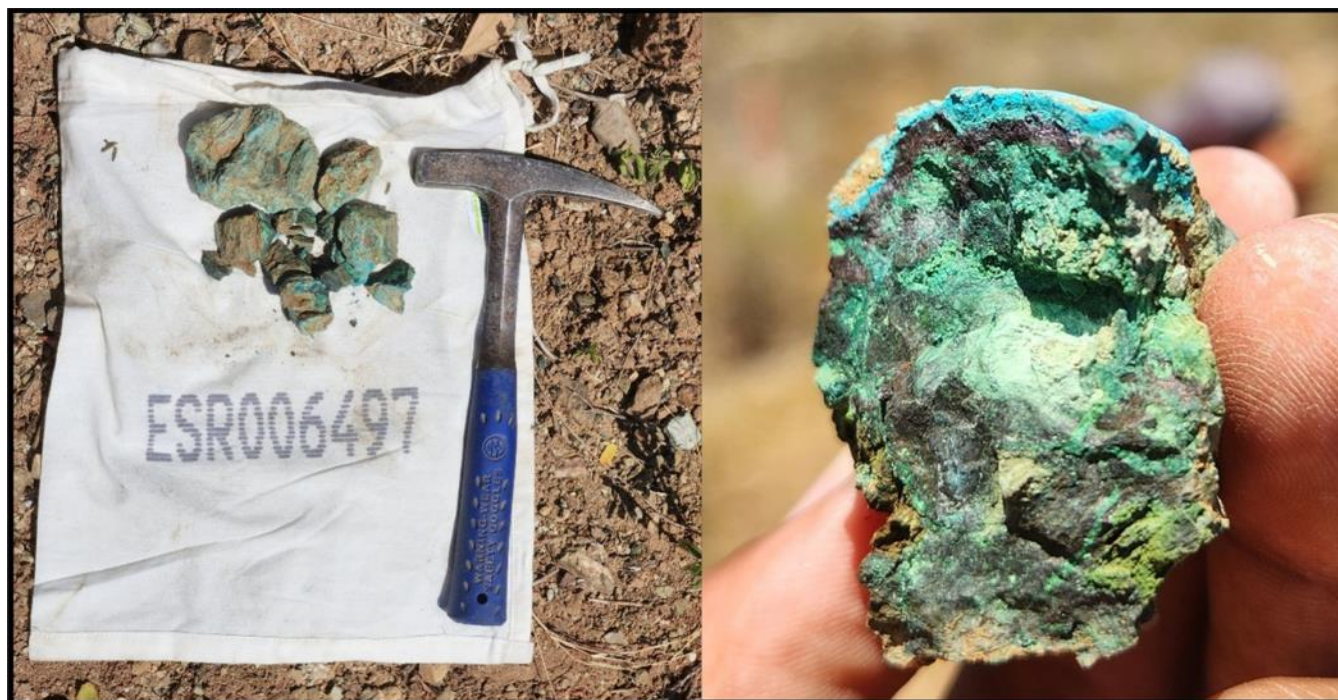
Figure 6: Sample ESR006497; left image shows exterior appearance, dominated by pale blue chrysocolla*, while the right image shows the chrysocolla is surface skin (1-2%) overlying an interior of bright green malachite (30-40%), brown goethite (40-50%), along with an unknown yellow-green mineral (~5%) and grey silica (5-10%).
