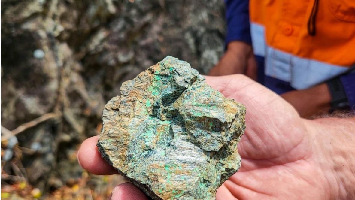
Figure 3: Example of copper mineralisation* within hydrothermally altered porphyritic rock, sampled as ESR0060498. The copper mineralisation consists of 1-2% malachite films on fracture surfaces of the rock mass.
