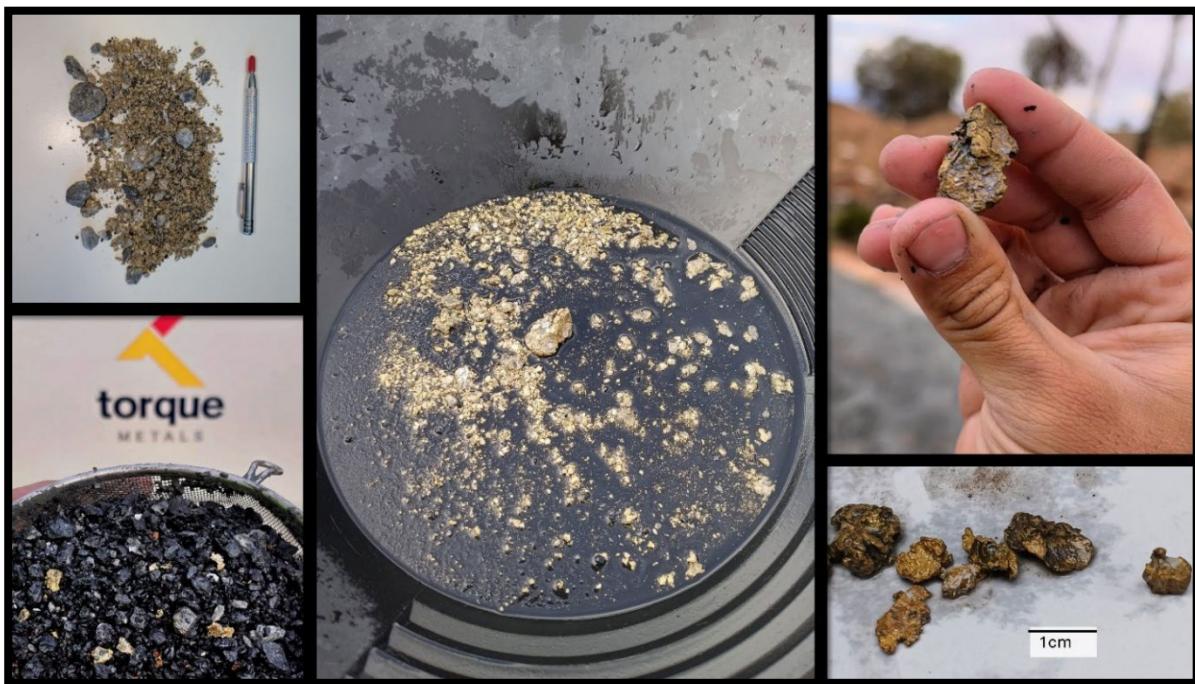
Figure 1: Various images of the panned gold nuggets and visible gold specimens from RC hole 26HRC135. The first three metres (122-125m) contained varying amounts of visible gold specimens with the interval from 123-124m (Photon assay result: 3,625g/t Au) containing the majority of the specimens in this figure. Torque is completing various QA/QC checks on the entire intercept (outlined below). Top Left: Total panned visible gold specimens collected from 122m-125m in 26HRC135.
