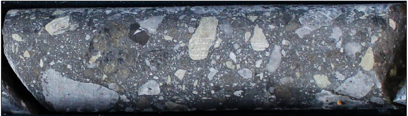
Figure 4 - High-grade breccia, core photograph of BAR034 3.55 m @ 9.01 AuEq from 63.70m
