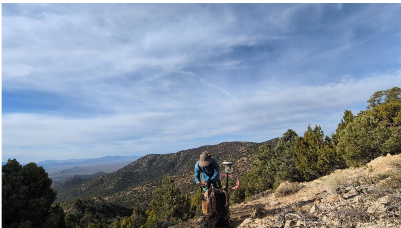
Figure 2: Zonge undertaking ground-gravity data acquisition at the Medicine Range Project.
