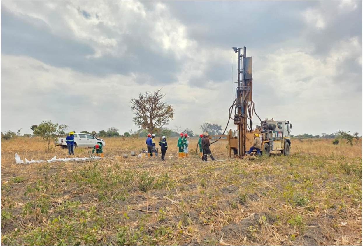
Figure 1. Aircore drilling in progress at the Mkanda Project in Malawi, Africa.
