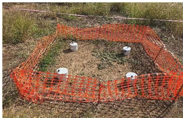
Figure 1: Example test cell with static chambers in situ at the NBRC Landfill site
