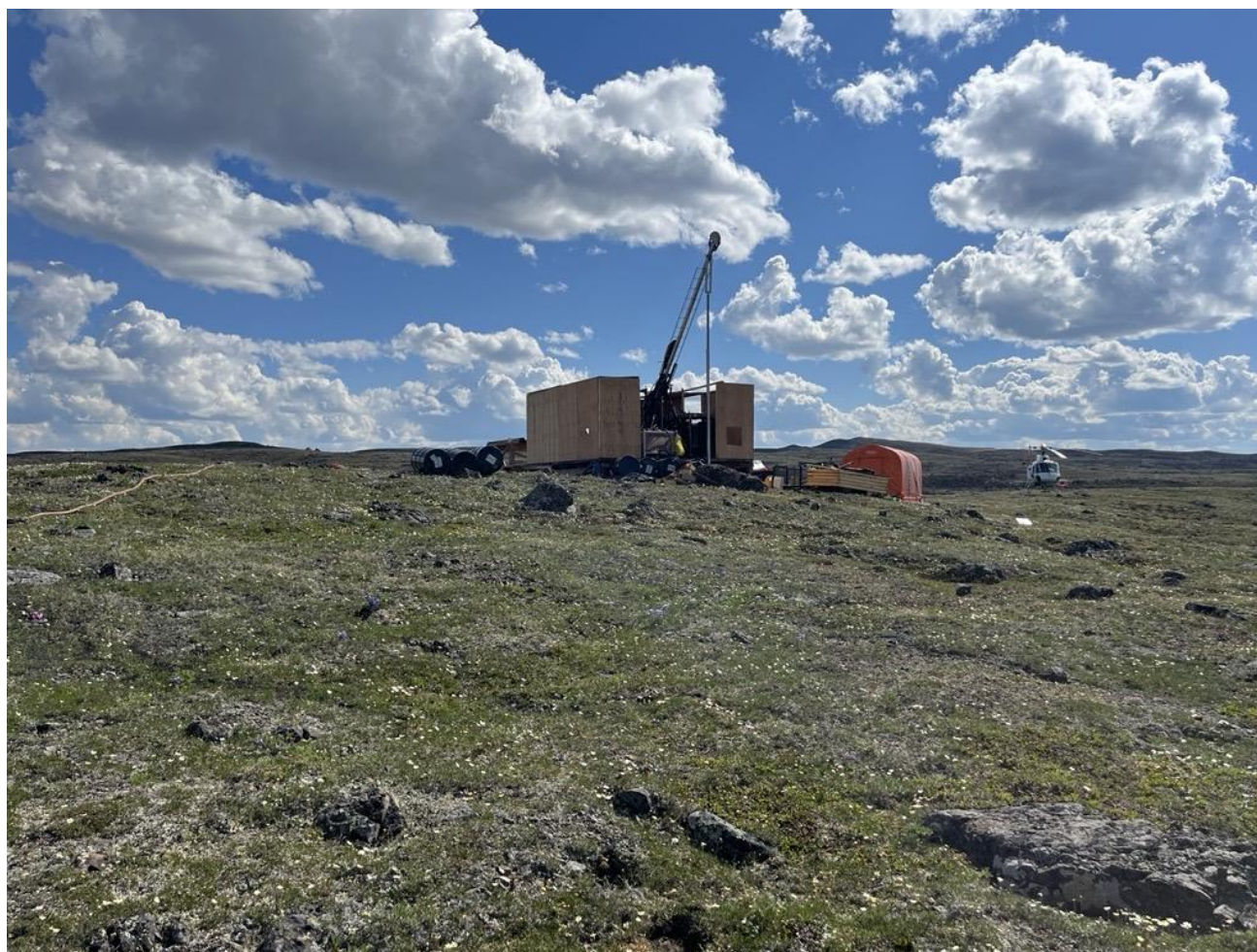
Figure 6 - Diamond drilling rig at DAN26027 along the north-eastern extension of Danvers 1.
