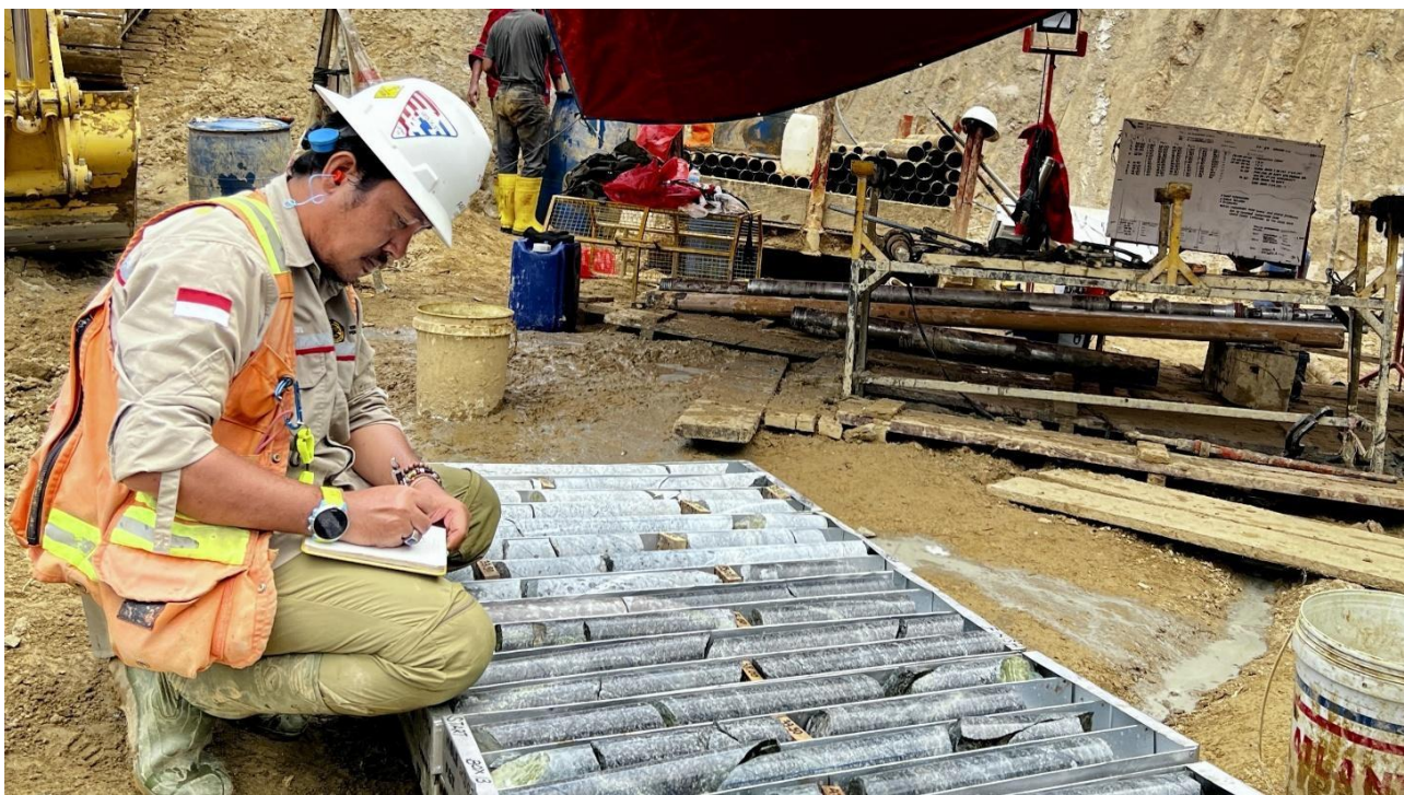
Figure 7: Geological logging of core at the Idenburg Gold Project, Papua, Indonesia.
