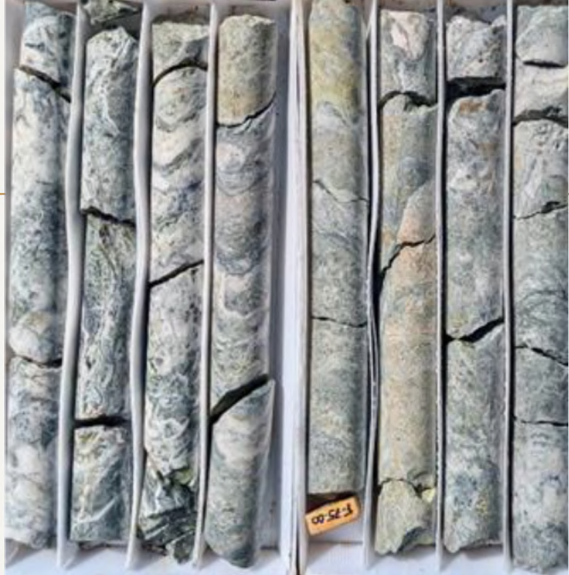
1 Banded quartz vein in drill core. CDH-152: 1.98m @ 4.59 g/t gold, 520 g/t silver from 18.5m (left) and CDH-154: 1.90m @ 1.83 g/t gold, 305 g/t silver from 75.1m (right).
