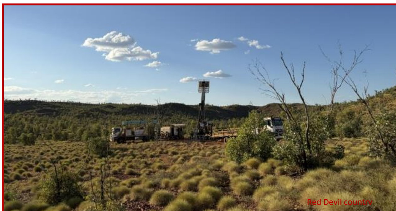
Image 1: Red Devil IP target diamond drilling underway by Terra Drilling.
