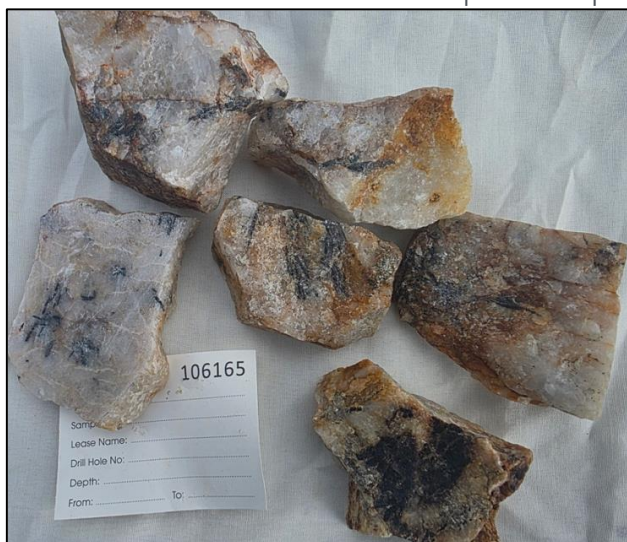
Figure 3 - Photo of Sample No:106165, FOV 15 cms. Location:189390mE 8027748mN. Milky white vein quartz included with abundant coarse wolframite blades to 3cm, weak iron staining, Assay: 5.46% W
