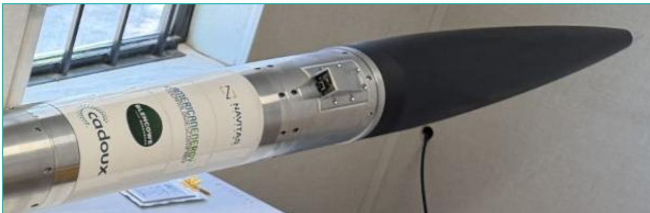
Nose cone and Control Management Stage of the Navitas Pluto rocket – Flight 008.
