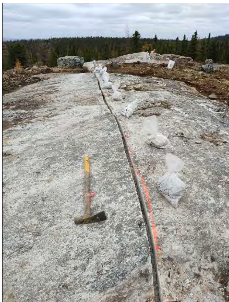
Figure 3-10 Channel sampling at Spodumene Mountain (source: WhiteRock, 2023)
