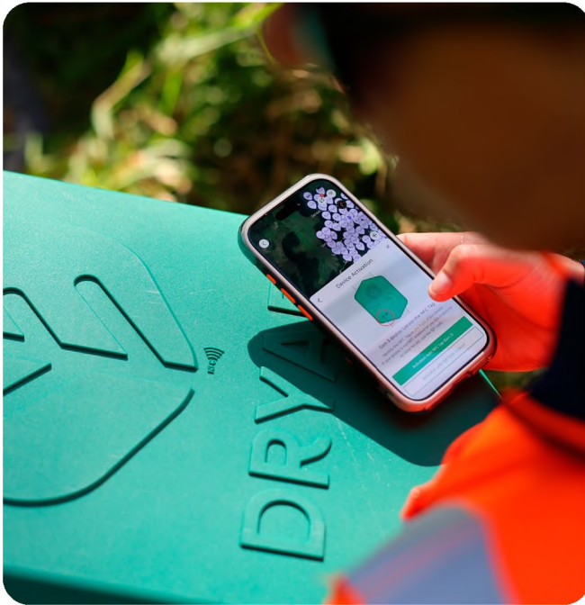
A fire-detection, solar-powered IoT sensor at Waitangi Endowment Forest.
