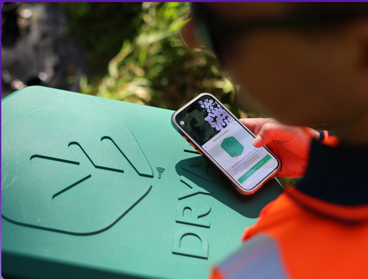
A fire-detection, solar-powered IoT sensor at Waitangi Endowment Forest.
