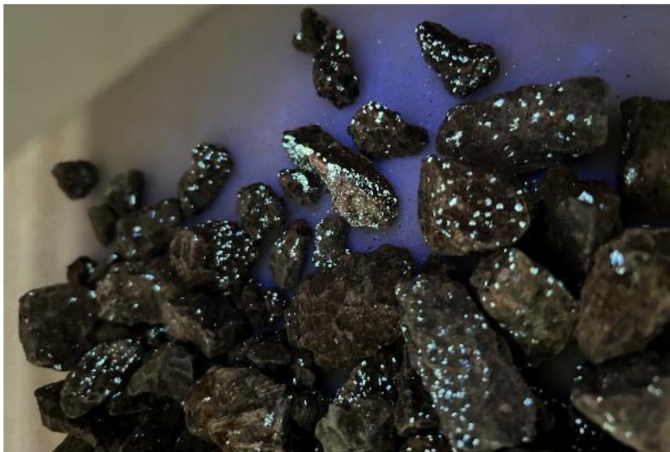
Figure 1; High grade sorted fraction (Set 1) from the Conquest Pit sample LKMET0006 under ultraviolet light, showing characteristic blue-white fluorescence of scheelite. This fraction returned an assay of 1.91% WO 3 , approximately 3.1x the calculated raw feed grade (refer Table 1).
