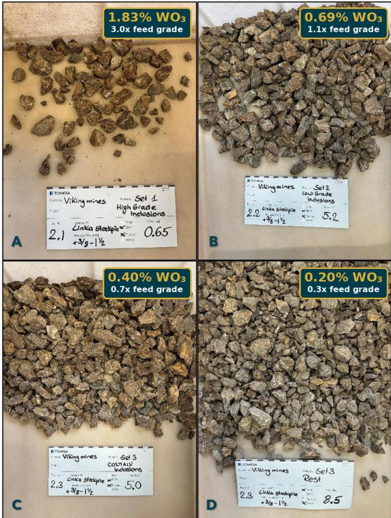
Figure 3; TOMRA XRT sorted fractions from the Linka Stockpile sample with assayed grades: A: Set 1 High Grade Inclusions (1.83% WO 3 ), B: Set 2 Low Grade Inclusions (0.69% WO 3 ), C: Set 3 CONTAIN™ Inclusions (0.40% WO 3 ) and D: Low-grade (0.20% WO 3 ) (clockwise from top left).
