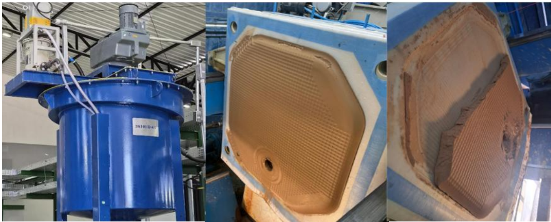
Figure 14: Solid liquid separation thickeners and residue filter MREC.
