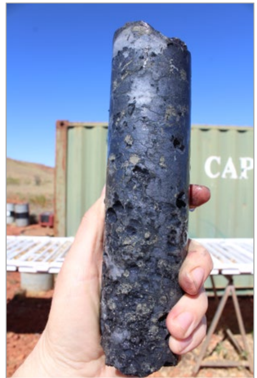
Photo 2 - Semi-massive pyrite – chalcocite mineralisation from 409.1 to 410.6m in ETG0226
