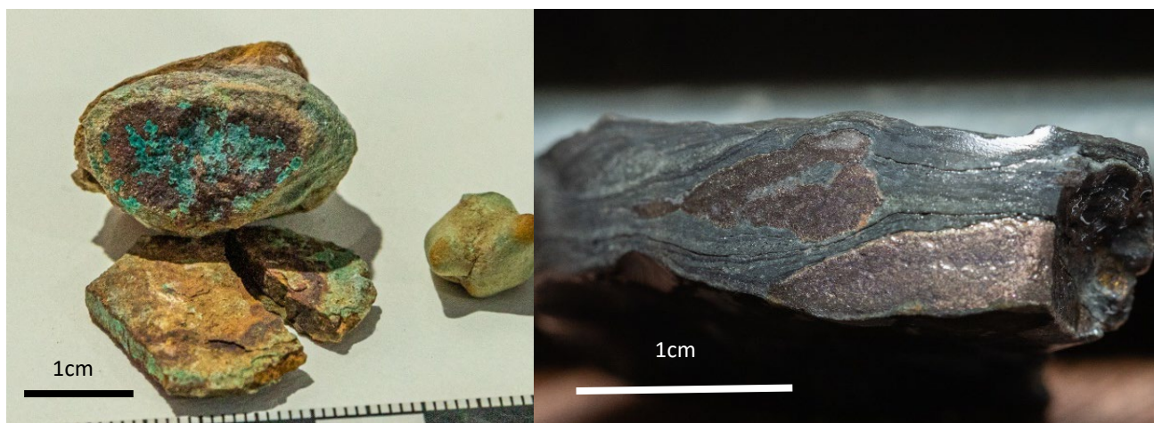
Photo 3 (left) – weathered copper rich nodules collected from surface at Area 1 (refer Figure 6) - containing malachite (interpreted after bornite-chalcocopyrite), visual estimate 10% malachite in 2.5cm diameter nodule Photo 4 (right) – primary copper rich nodule from historical drillhole (Mt Skinner DDH3 203.3m) located adjacent to Area 4 (refer Figure 6) containing bornite-chalcocopyrite, visual estimate 30% bornite-chalcocopyrite over ~1cm width. 10
