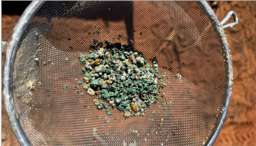
Photo 1: Recent drill hole EPT 2439 Copper Oxide Mineralisation (Malachite) at 46-47m (part of 2m @ 1.7% Cu)
