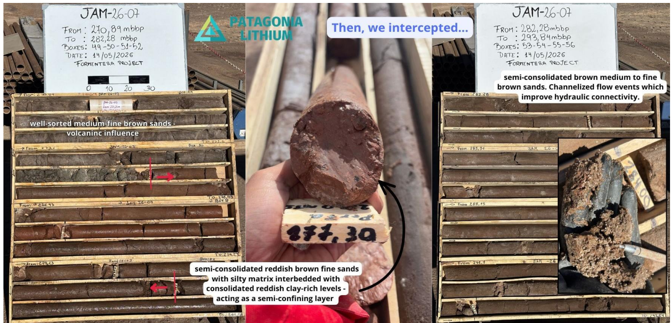
Figure 1. JAM 26-07 core sample 270m to 293m gravels and sand contributing to high porosity.
