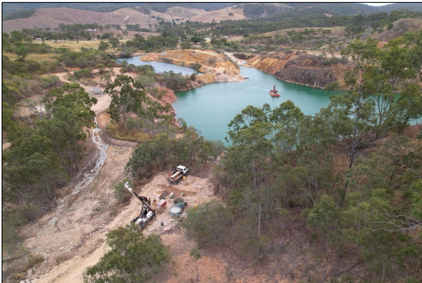
Figure 2 – Aerial picture of rig 12 & 19 drilling from a barge in the historic open pit.
