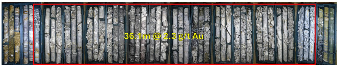
Figure 4: Erak Prospect, drillhole ERDD006 core photos (PQ diameter) with marked strong "phyllitic" (quartz-sericite-pyrite) alteration zone 36.1m @ 2.3 g/t Au from 51.8m drilling depth.
